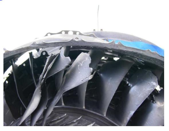
US Airways Flight 1549 - January 15, 2009 - Airbus A320 - double engine failure after collision with flock of geese (*Branta canadensis*)
